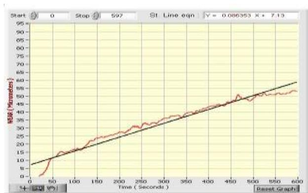
Figure 9 Wear test graph of sample1, at 3kgs load
