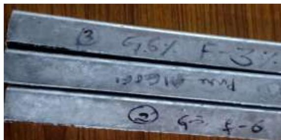
Figure 1 Casted Composite Samples
