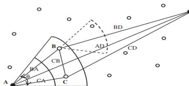
**Fig. 2:** FBR routing protocol illustration: the node in the transmitter cone y are candidate relays.
