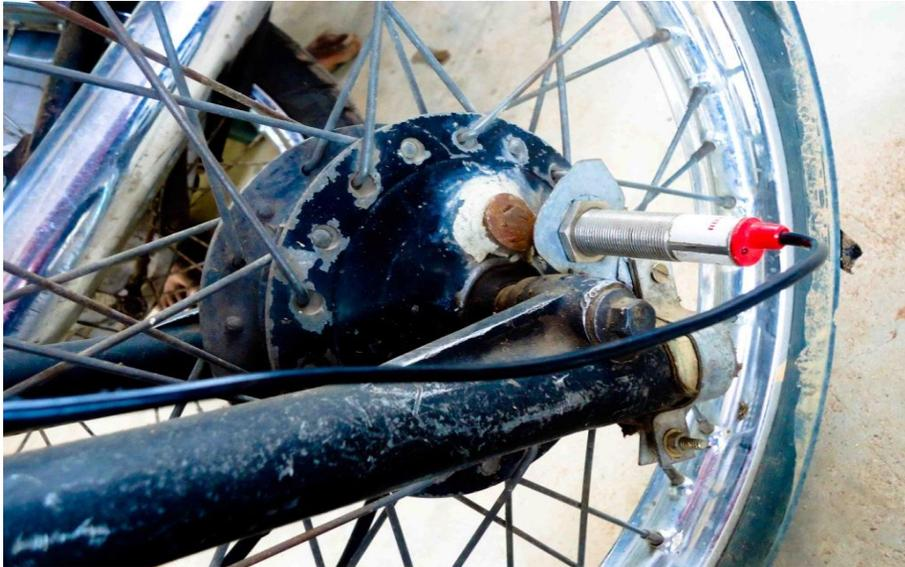
Fig. 14: Inductive speed sensor mounting
