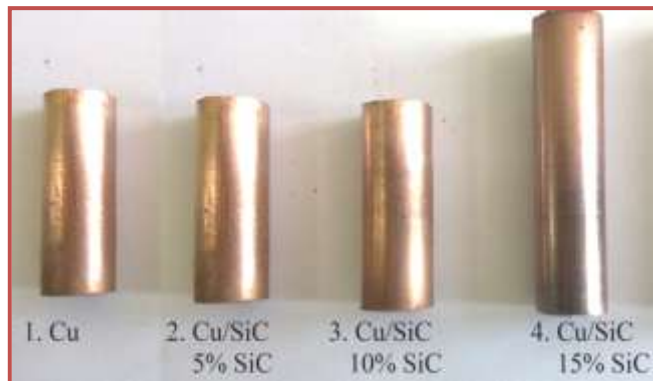
Fig. 6 Sintered composite tool electrodes
