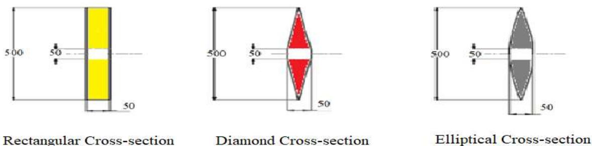
Figure 1. Cross-sections of the flywheel
