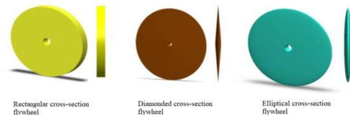
Figure 2. Parametric models of flywheel
