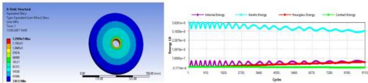
Figure5. *Stress distribution and Kinetic energy graph for Rectangular cross-sectioned flywheel with Graphene*
