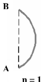
The first mode shape of a Simply-supported beam
