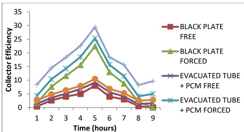
Figure 2. The variation of collector efficiency with time
