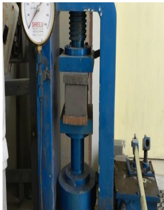
Figure 2: Compressive strength test
