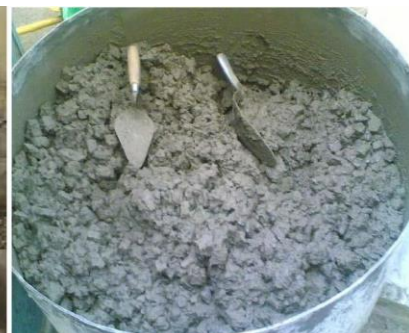
Figure 1. Rubber Aggregates Size of 4.12 mm Figure 2 Concrete Mixing using a Pan Mixer
