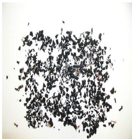
Figure 1. Rubber Aggregates Size of 4.12 mm Figure 2 Concrete Mixing using a Pan Mixer
