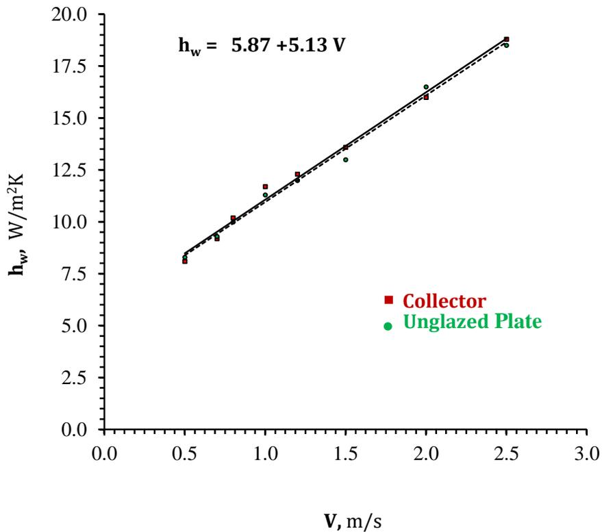
Figure 5: Deviation of  $h_w$  of Collector from that of Unglazed Plate
