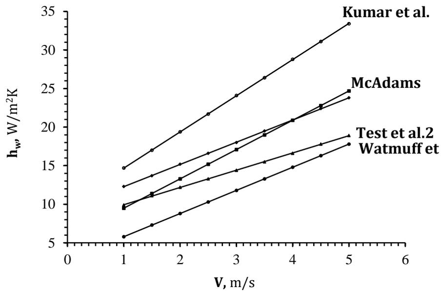
Figure 1:  $h_w$  at Various Wind Velocities from different Correlations
