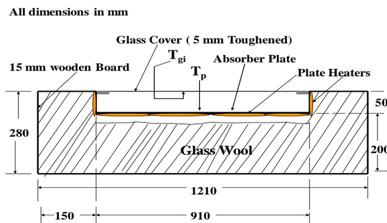
Figure 2: Indoor Experimental Single Glazed Collector
