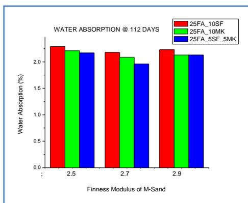
Fig 3. Water Absorption(%)@ 112 days
