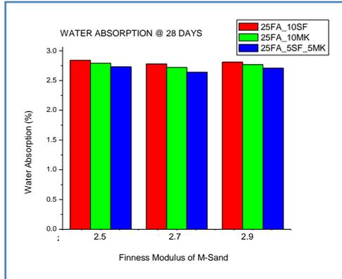
Fig 1. Water Absorption(%)@ 28days
