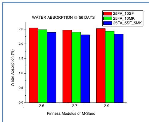
Fig 2. Water Absorption(%)@ 56 days
