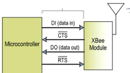
Fig: Interfacing Diagram of Zigbee.
