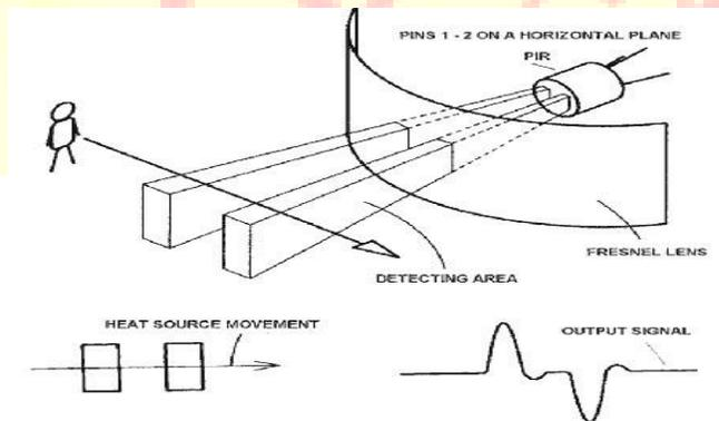
The PIR sensor itself has two slots in it, each slot is made of a special material that is sensitive to IR. We see that the two slots can 'see' out past some distance (basically the sensitivity of the
