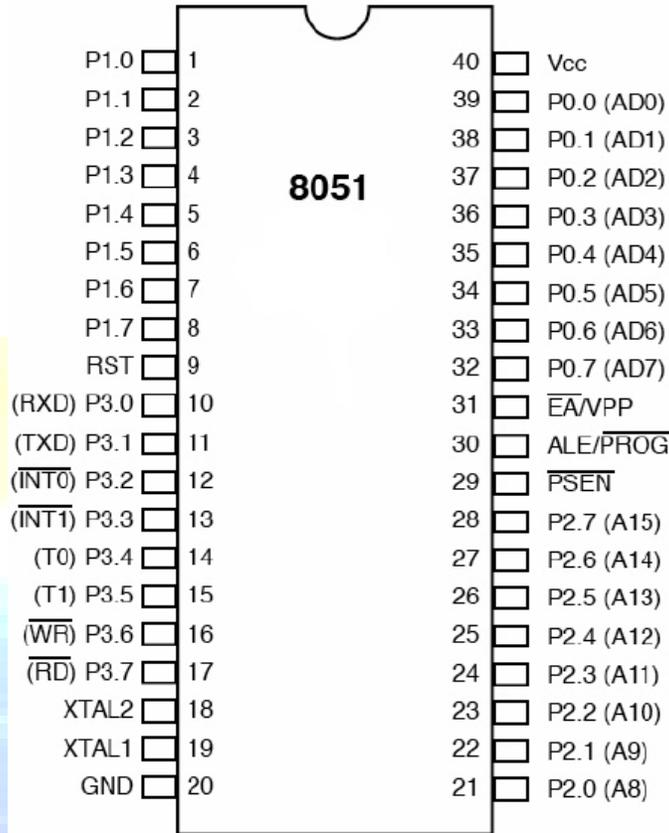
Fig: Pin Diagram of microcontroller 8051
