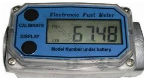
Fig1: Digital flow meter, reference from Google images
